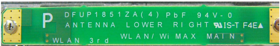
WLAN Main TX/RX Antenna
