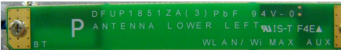
WLAN Aux TX/RX Antenna
