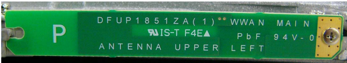
WWAN Main TX/RX Antenna
