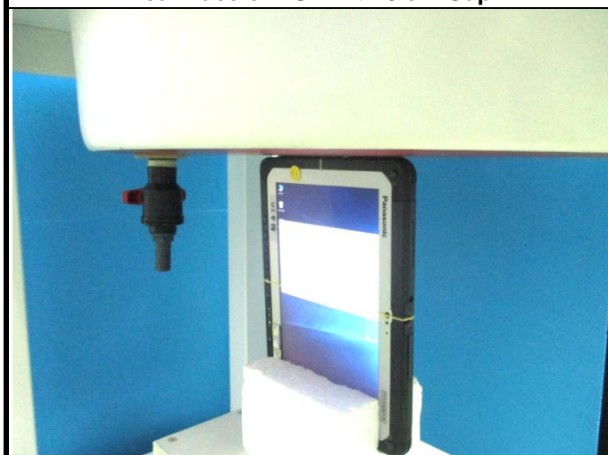
Left Side of EUT with 0 cm Gap
