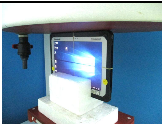
Top Side of EUT with 0 cm Gap
