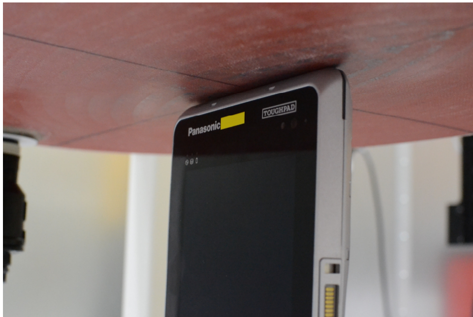
SAR Test Setup Photo 2: Top Edge (Perpendicular) at 0.0 cm
