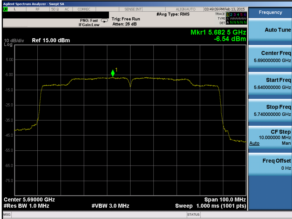
Plot 6-30. Power Spectral Density Plot (80MHz BW 802.11ac (UNII Band Gap) – Ch. 138)
