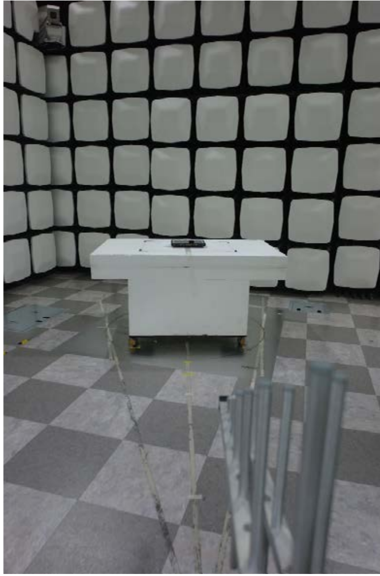
RFID Radiated Test Setup Photo for 30 MHz ~ 1 GHz :
