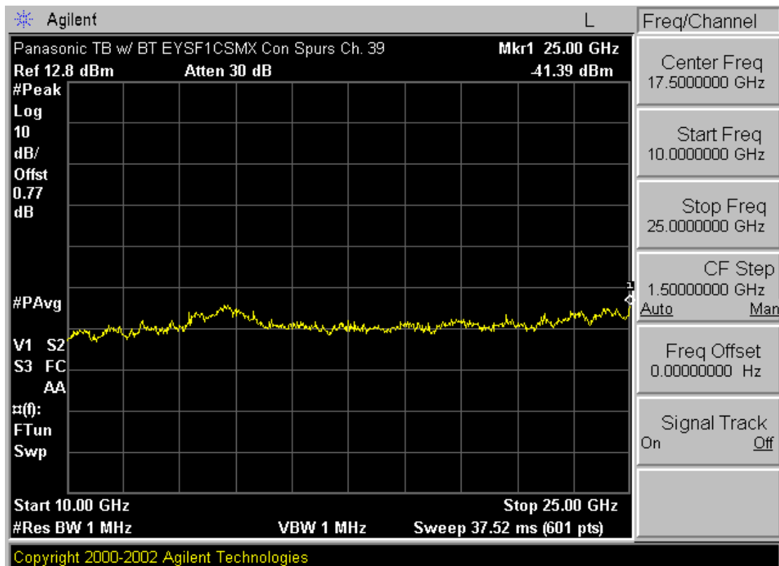
Plot 6-15. Conducted Spurious Plot (Bluetooth – Ch. 39)
