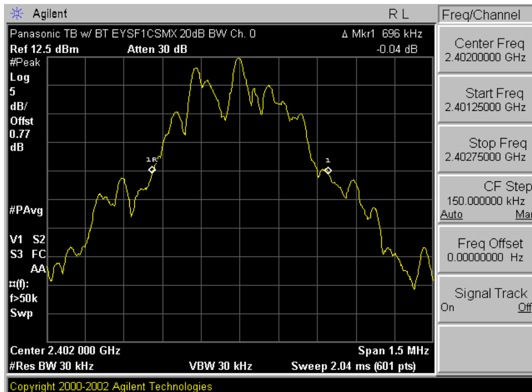
Plot 6-1. 20dB Bandwidth Plot (Bluetooth – Ch. 0)
