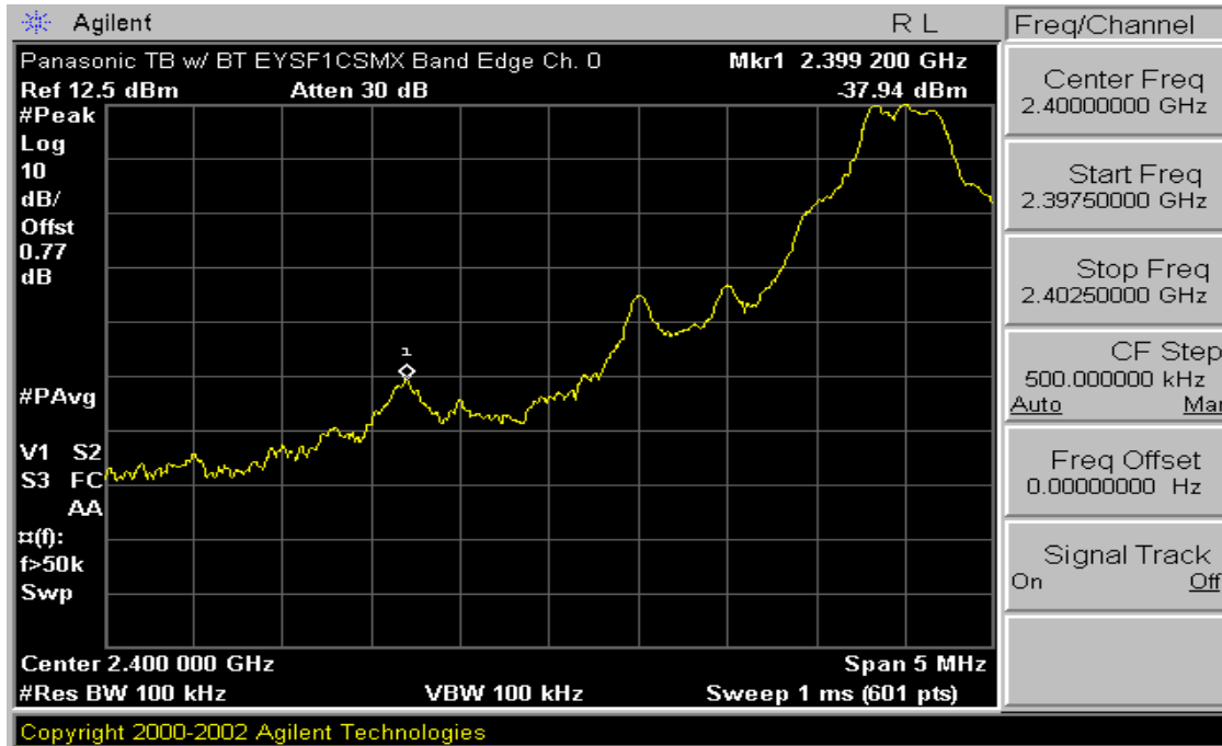
Plot 6-4. Band Edge Plot (Bluetooth – Ch. 0)
