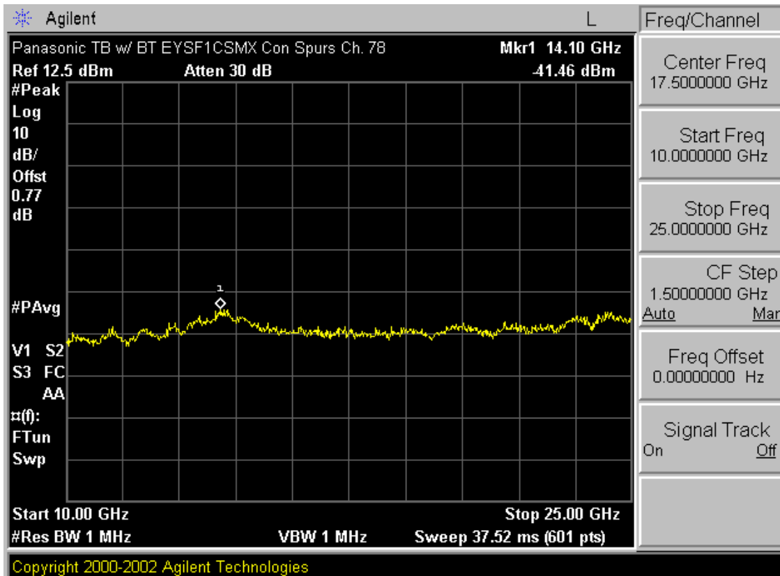
Plot 6-18, Conducted Spurious Plot (Bluetooth – Ch. 78)
