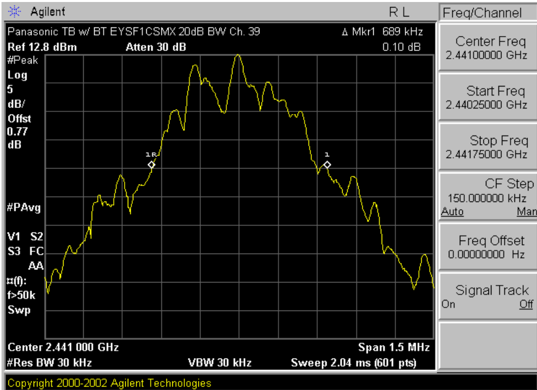
Plot 6-2. 20dB Bandwidth Plot (Bluetooth – Ch. 39)
