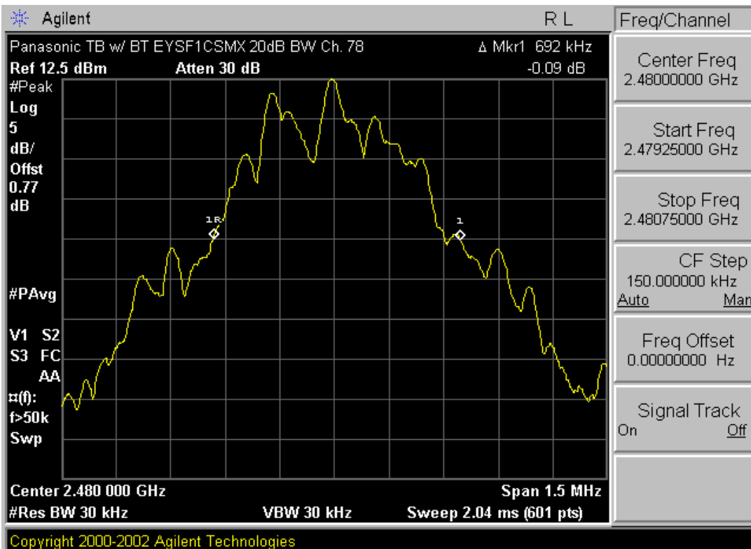
Plot 6-3. 20dB Bandwidth Plot (Bluetooth – Ch. 78)
