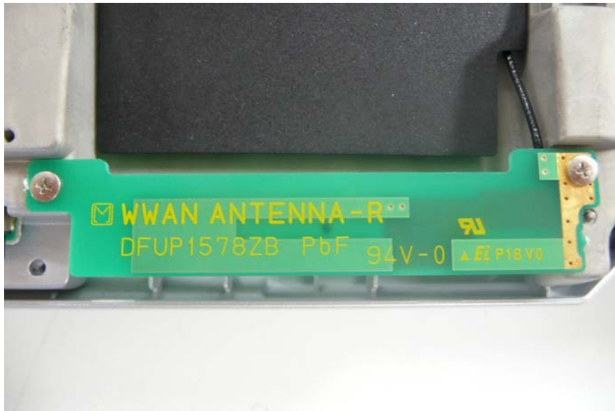
HSDPA Main TX/RX Antenna
