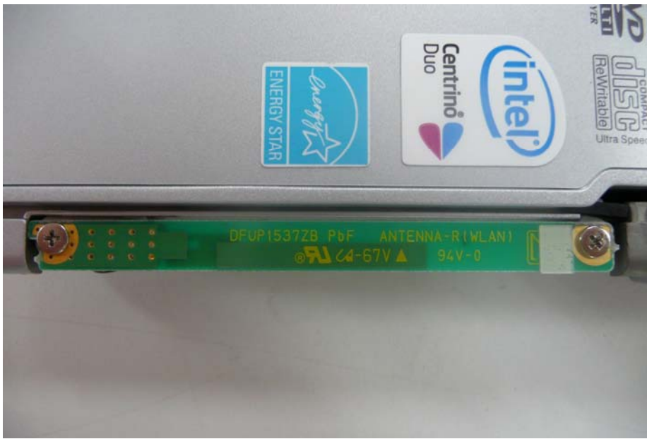
WLAN Main TX/RX Antenna
