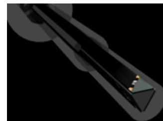
Figure 4-3 Triangular Probe Configuration
