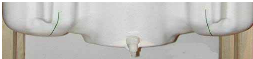
Figure 7-2 SAM Twin Phantom Shell
