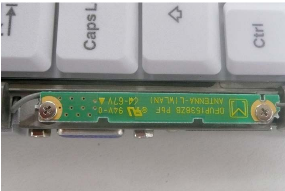
WLAN AUX TX/RX Antenna
