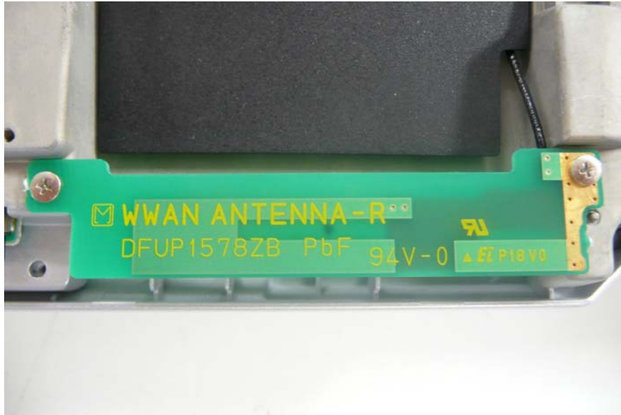
EVDO Main TX/RX Antenna
