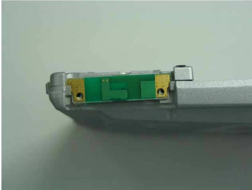
Main TX/RX Antenna magnified View
