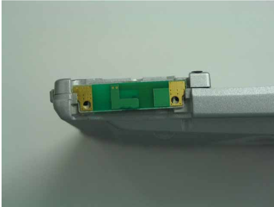
Main TX/RX Antenna magnified View
