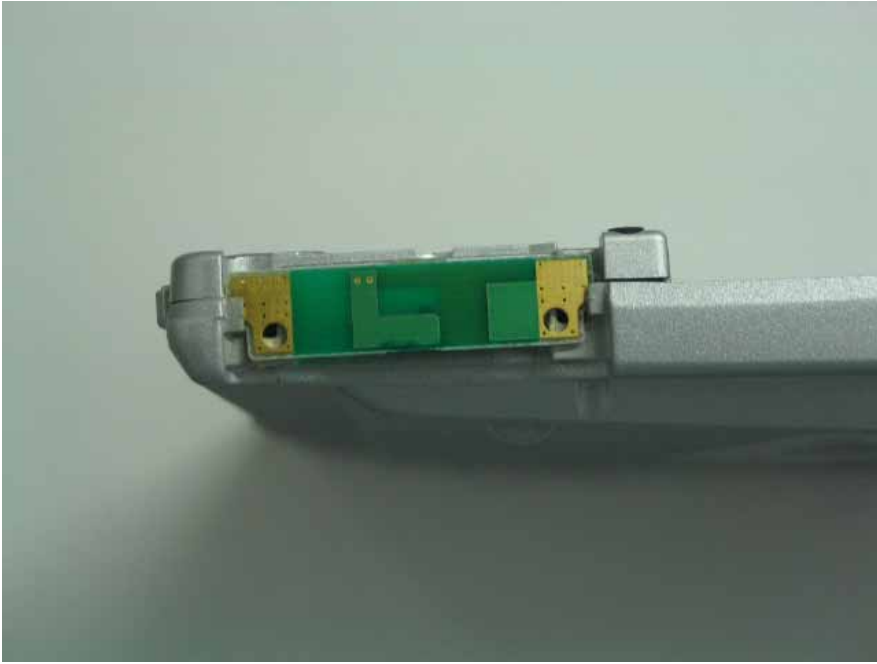
Main TX/RX Antenna magnified View
