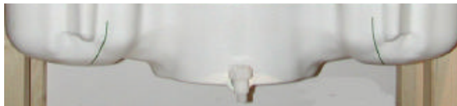
Figure 7.2 SAM Twin Phantom shell
