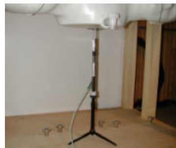
Figure 12.1 Dipole Validation Test Setup
