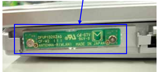
Main TX/RX Antenna Magnified View
