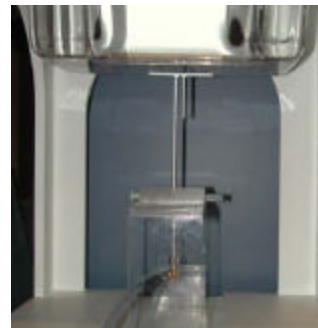
Figure 10.1 Dipole Validation Test Setup
