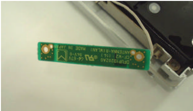
Right Antenna Top View
