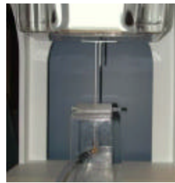
Figure A.0 Dipole Validation Test Setup
