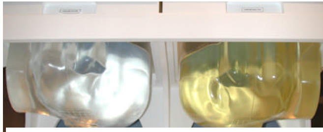
Figure 7.1 Left and Right SAM Phantom shells
