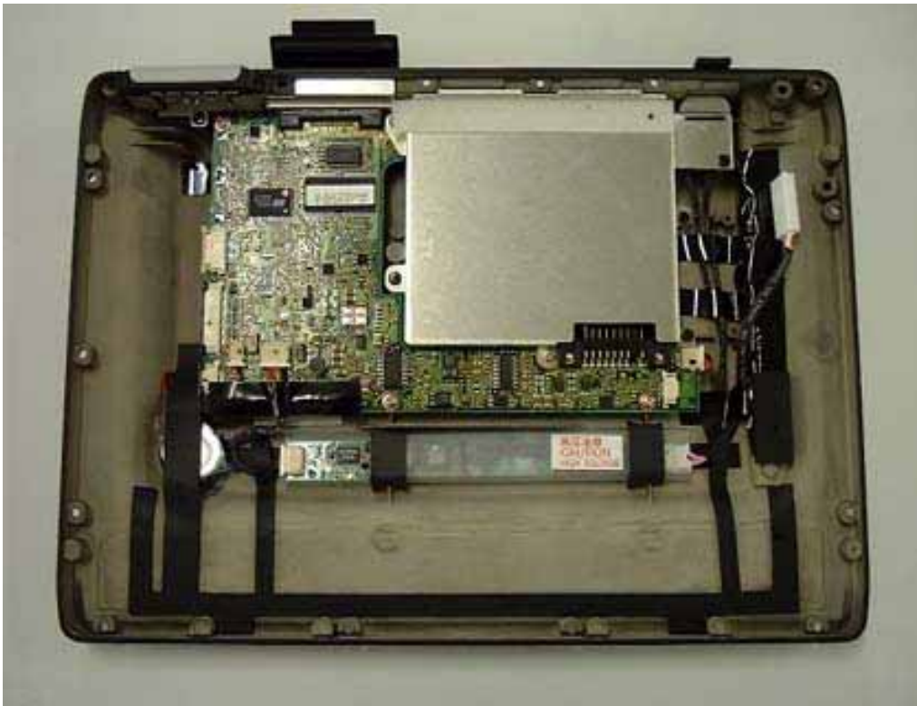
CF-VDW07 Inside View (Bottom Cover open)
