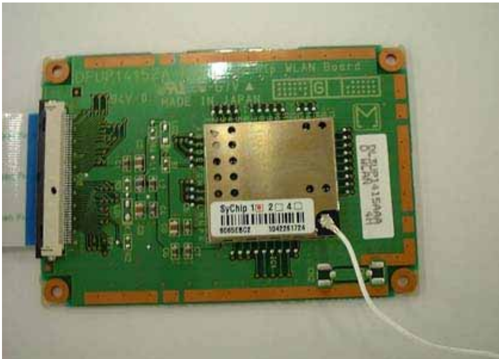
WLAN module (SyChip) on Daughter Board
