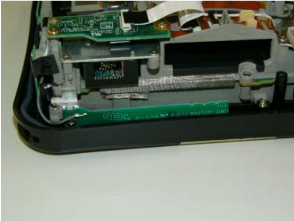
WWAN Main TX/RX Antenna
