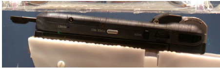
Figure 8-2 CompactFlash radio card in PDA host configuration
