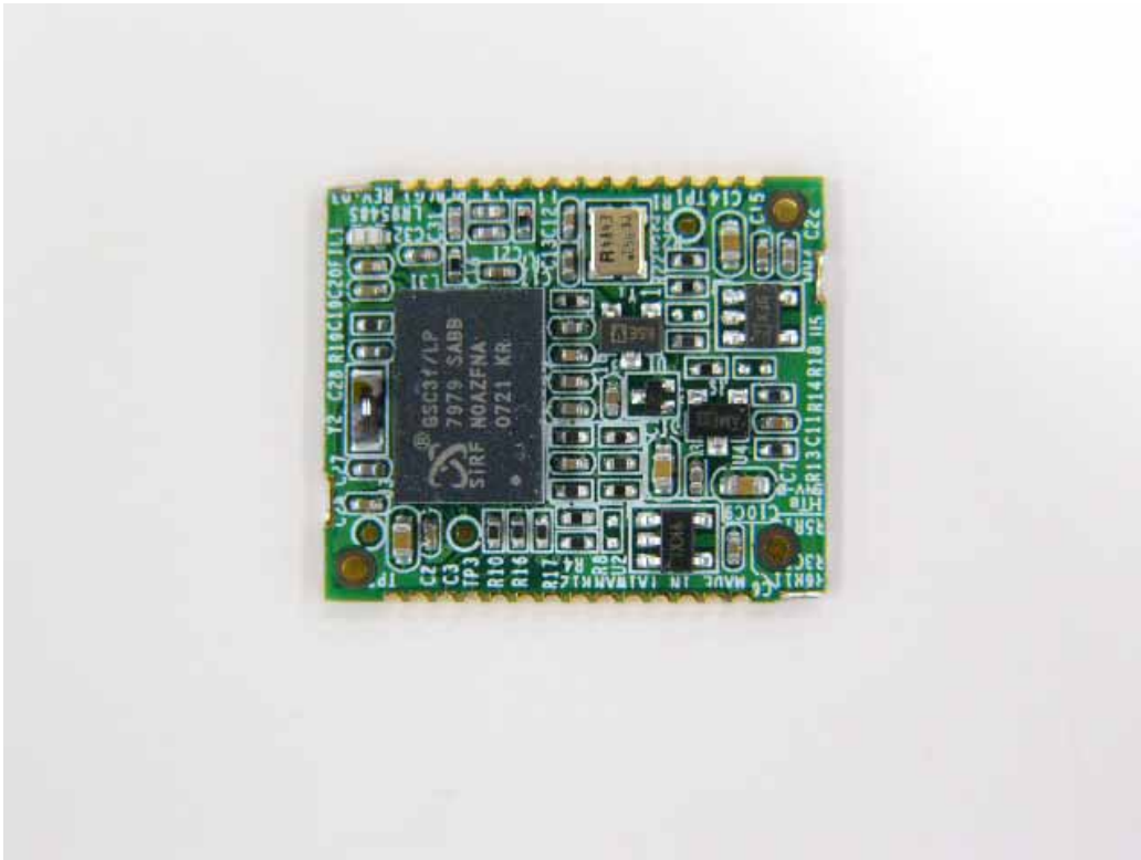
GPS Module inside Top View
