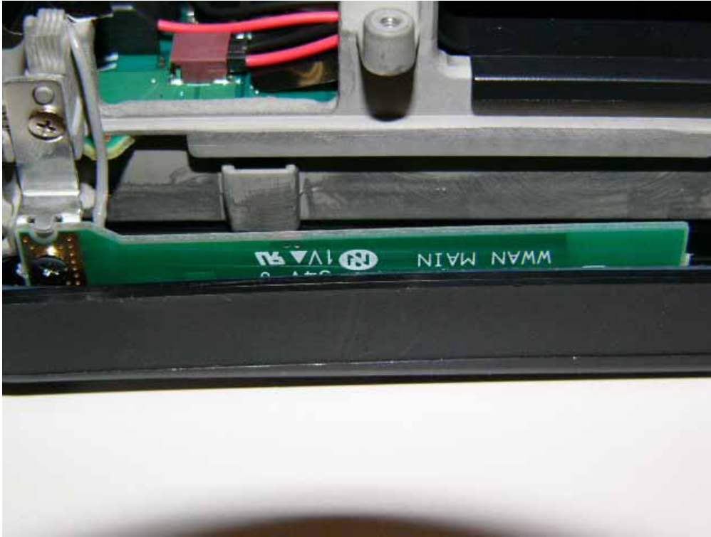
WWAN Main TX/RX Antenna
