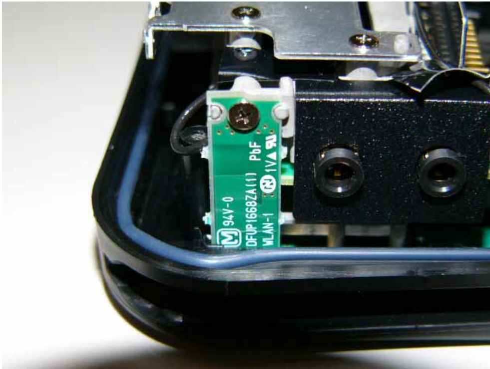
WLAN Main TX/RX Antenna
