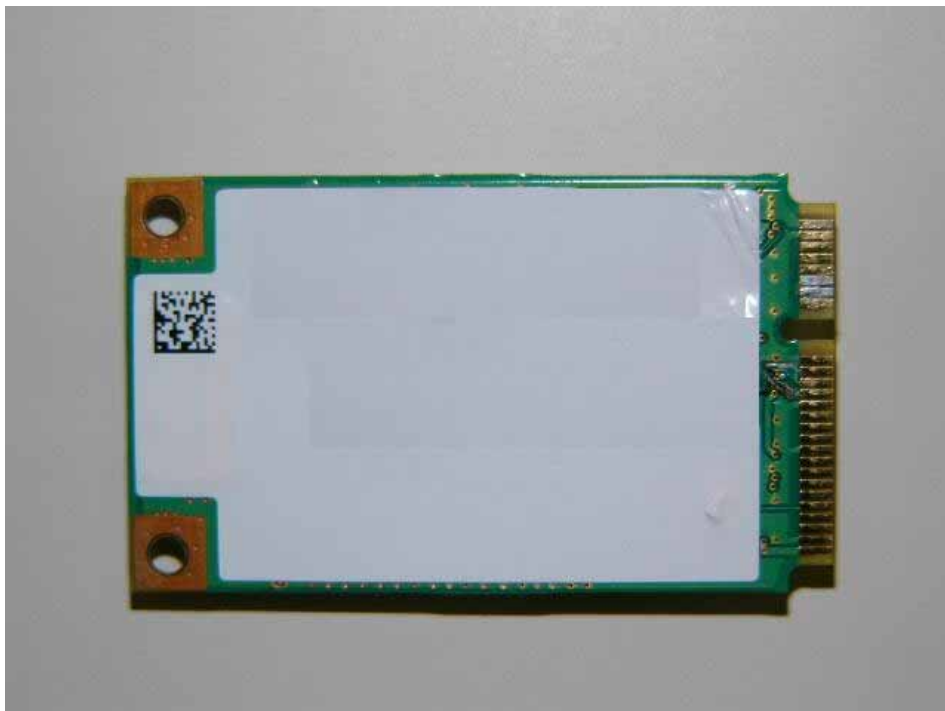
WLAN Exterior Bottom View
