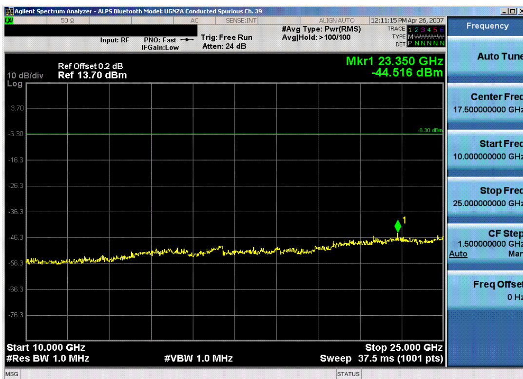
Plot 6-15. Conducted Spurious Plot (Bluetooth – Ch. 39)
