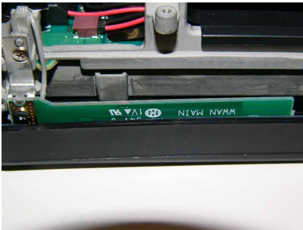
WWAN Main TX/RX Antenna
