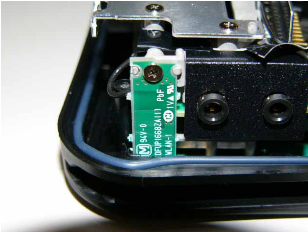
WLAN Main TX/RX Antenna
