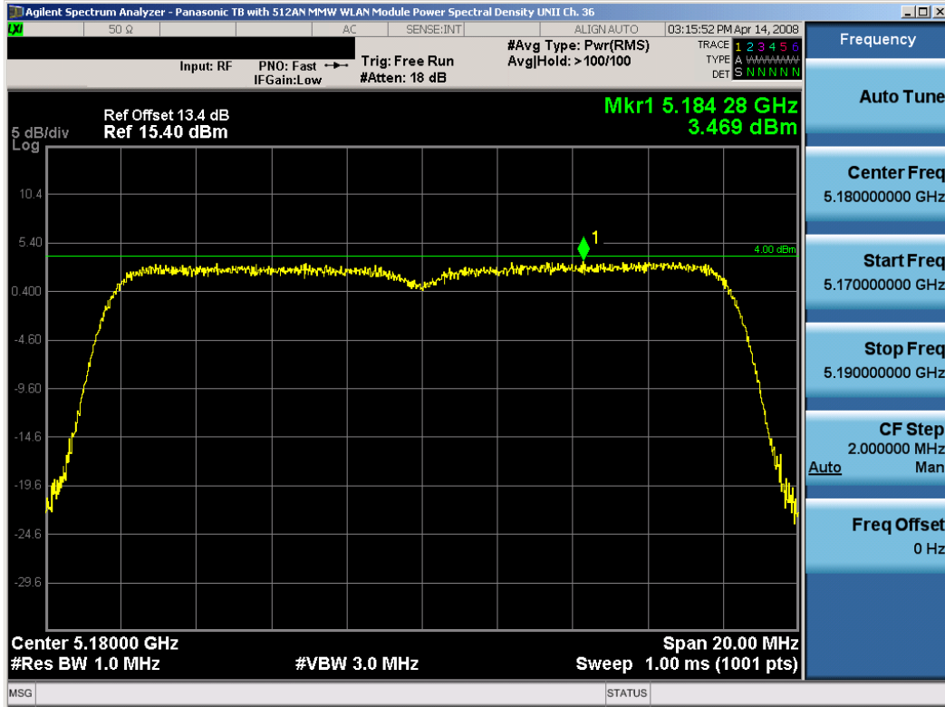
Plot 6-11. Peak Power Spectral Density Plot (802.11a (UNII) – Ch. 36)
