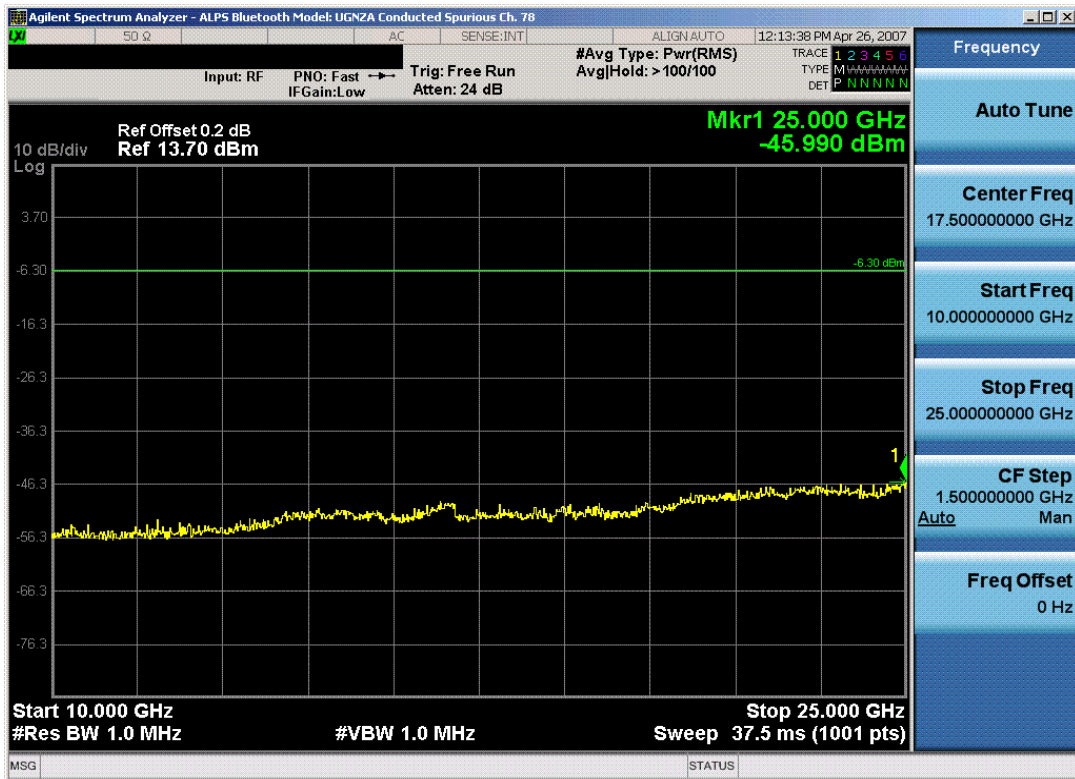
Plot 6-17. Conducted Spurious Plot (Bluetooth – Ch. 78)
