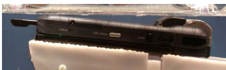
Figure 8-2 CompactFlash radio card in PDA host configuration
