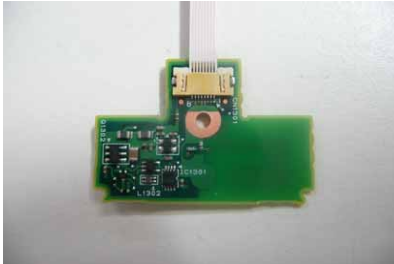
Bluetooth Card inside Top View
