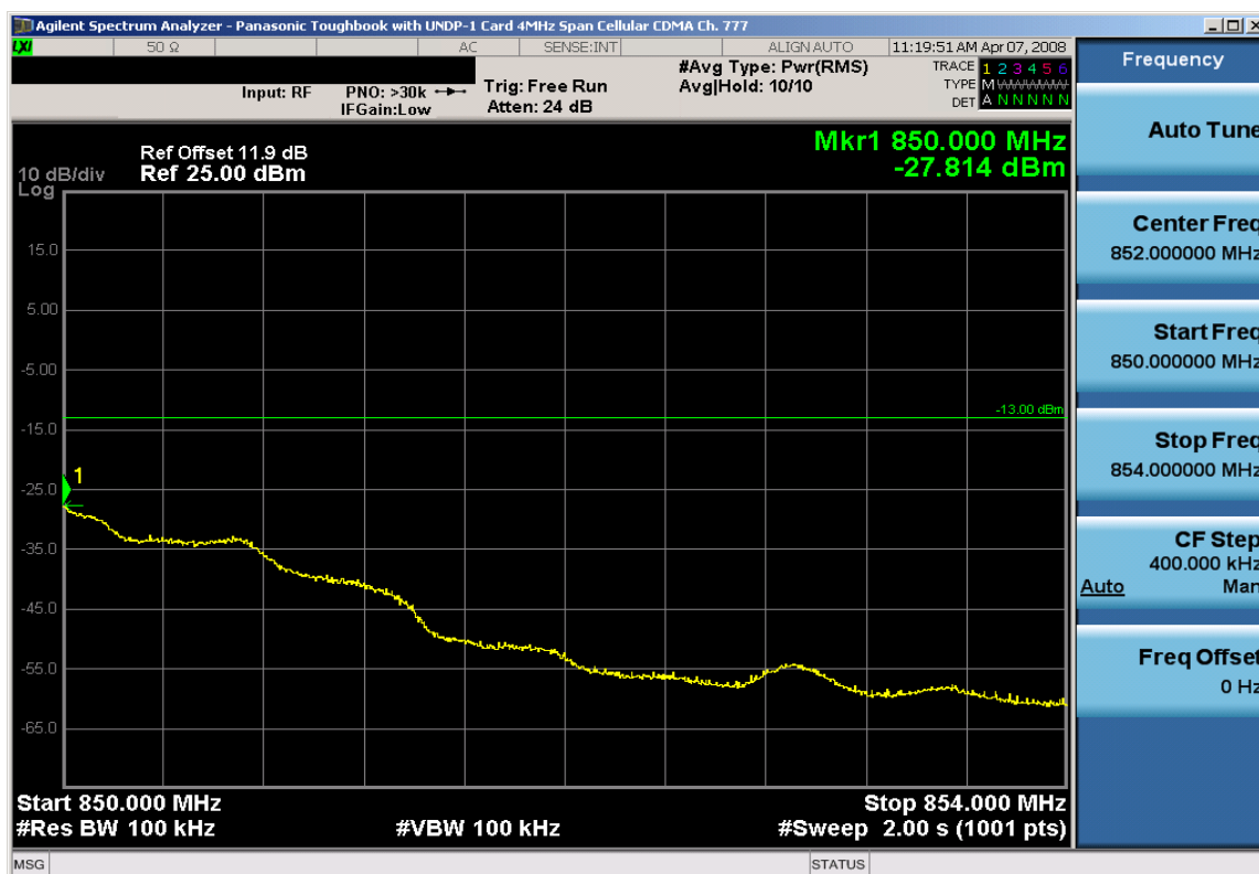
Plot 7-56. 4MHz Span Plot (Cellular CDMA Mode – Ch. 777)
