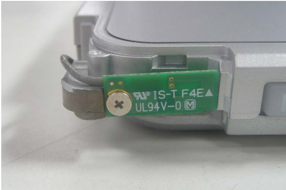
Main TX/RX Antenna Magnified View
