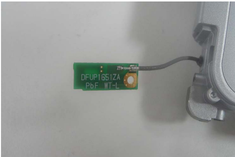
Main TX/RX Antenna Magnified View(Reverse side)
