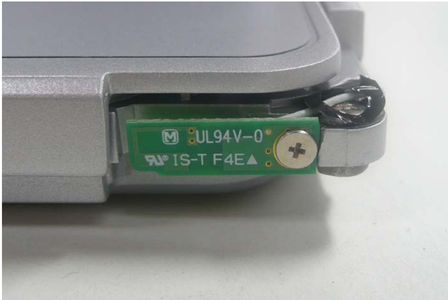
Aux TX/RX Antenna Magnified View
