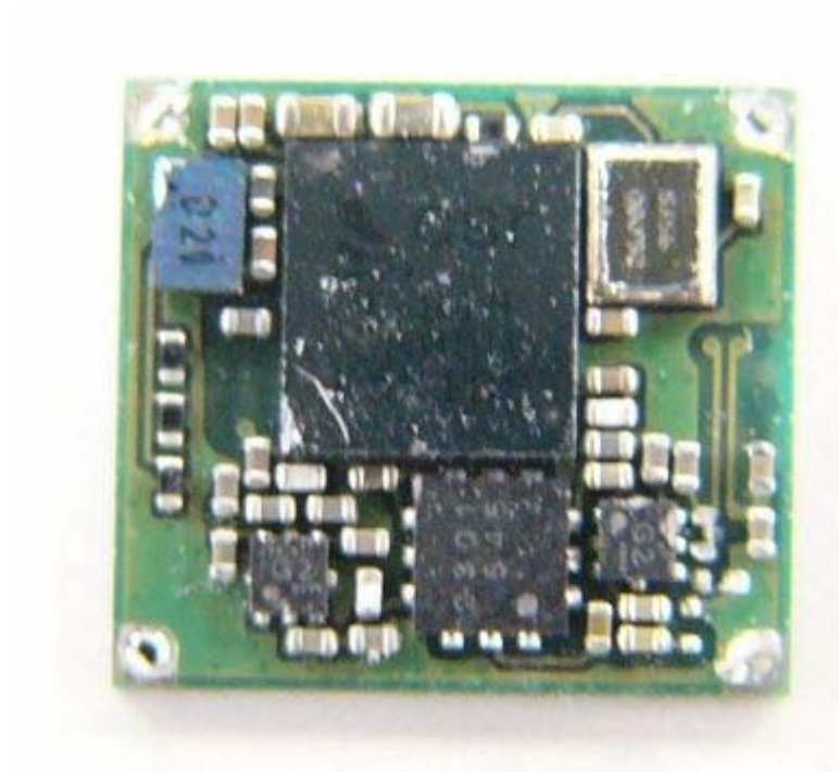
BlueTooth Module inside Top View
