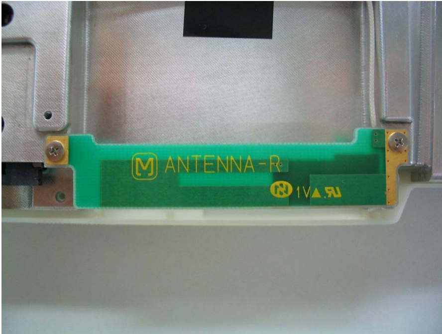
EVDO Main Antenna Magnified Viwe
