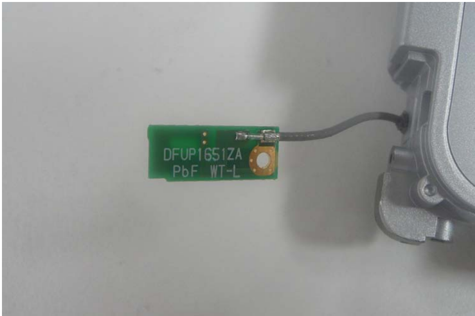
Main TX/RX Antenna Magnified View(Reverse side)
