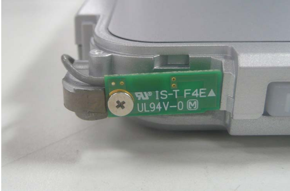
Main TX/RX Antenna Magnified View
