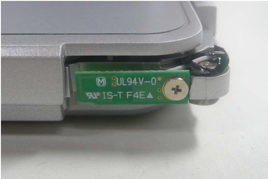
Aux TX/RX Antenna Magnified View
