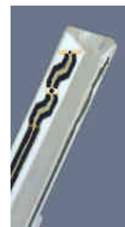
Figure 3.2 Probe Thick-Film Technique
