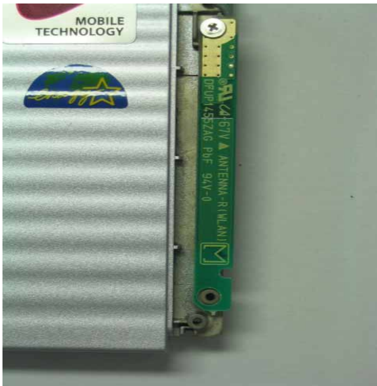
Main TX/RX Antenna magnified View
