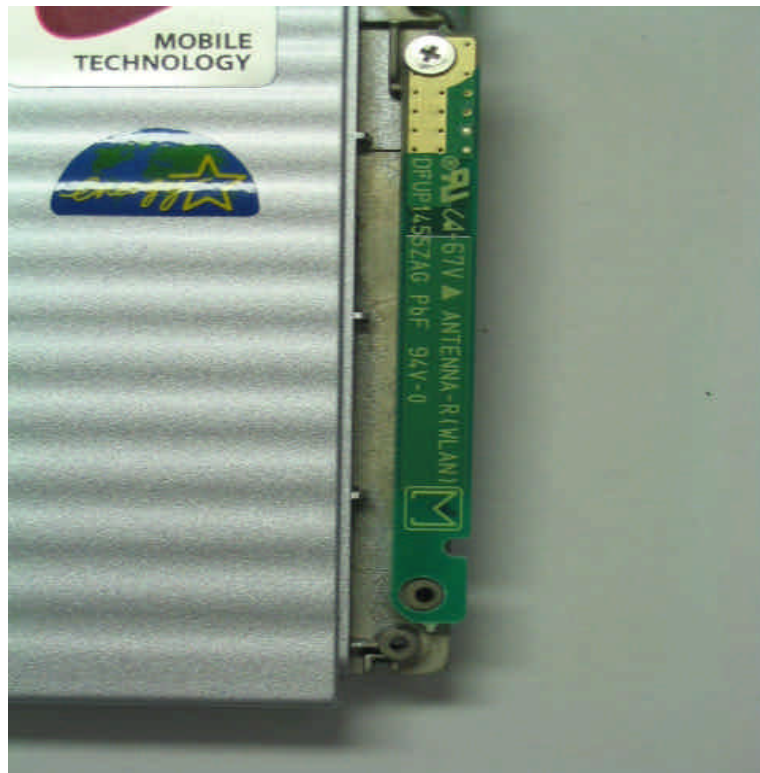
Main TX/RX Antenna magnified View
