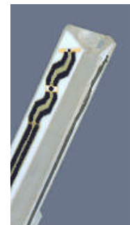
Figure 3.2 Probe Thick-Film Technique
