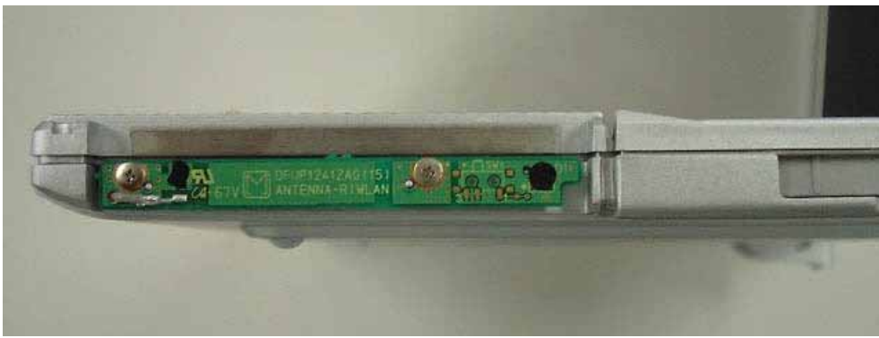
Main TX/RX Antenna magnified View
