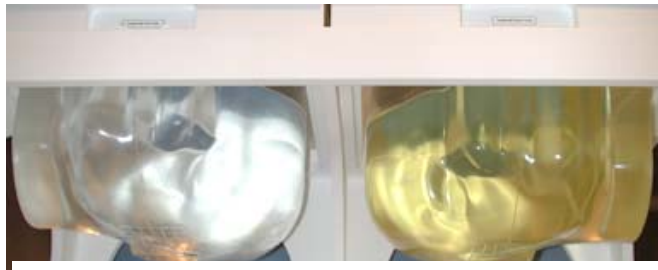
Figure 7.1 Left and Right SAM Phantom shells
