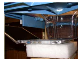
Figure 14.2 Body SAR Test Setup
