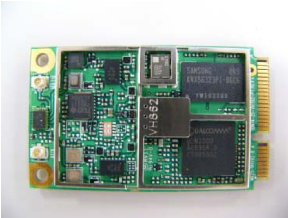
WWAN Module Interior Top View
