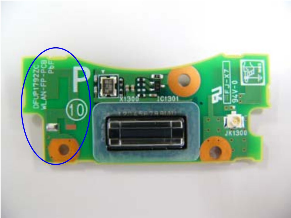
Bluetooth TX/RX Antenna (separated type: Top)
