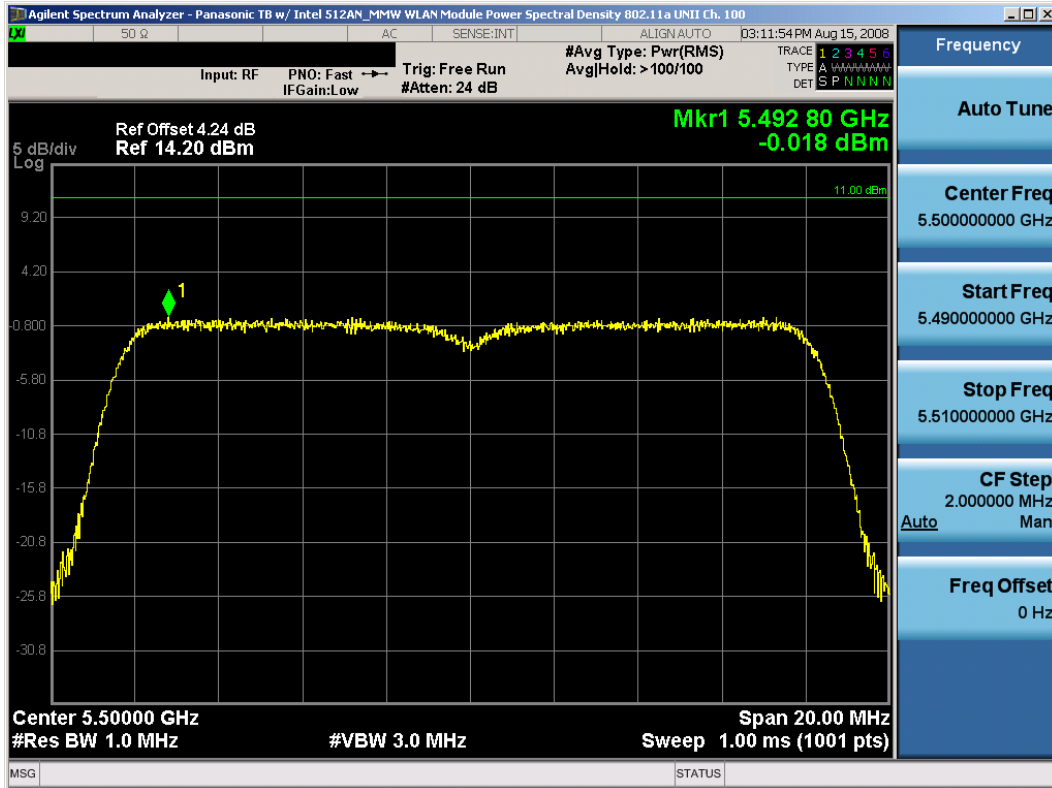
Plot 6-23. Peak Power Spectral Density Plot (802.11a (UNII) – Ch. 100)
