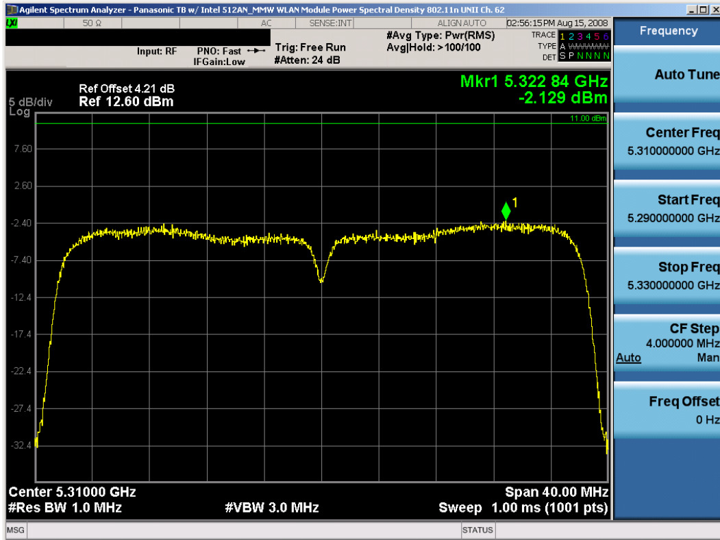
Plot 6-29. Peak Power Spectral Density Plot (802.11n (UNII) – Ch. 62)
