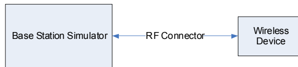
Figure 12-1 Power Measurement Setup
