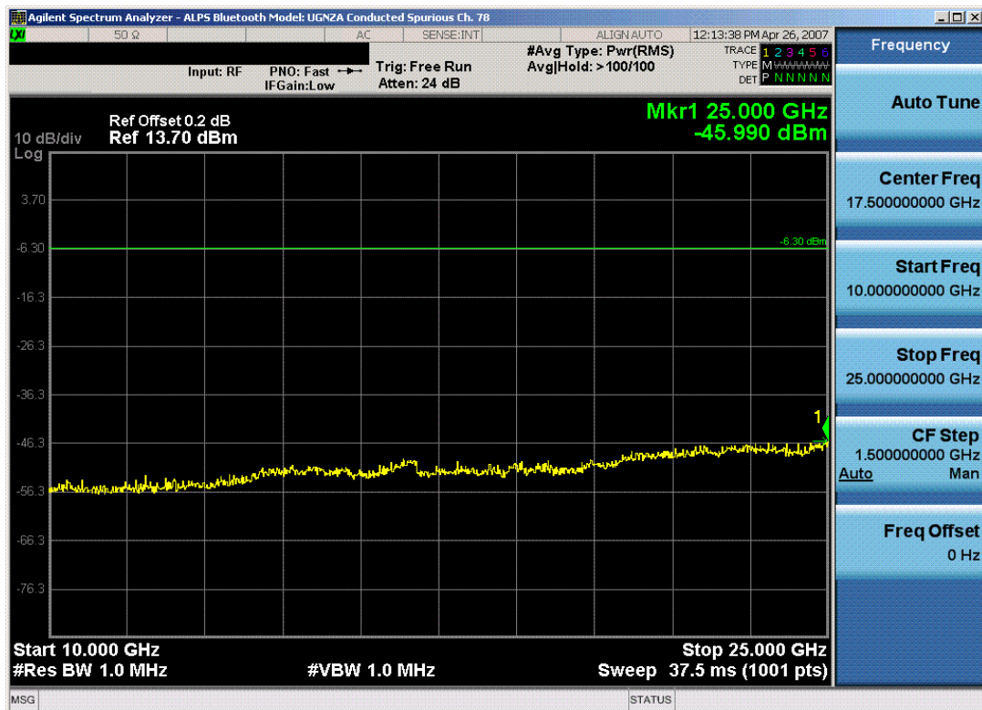
Plot 6-17. Conducted Spurious Plot (Bluetooth – Ch. 78)
