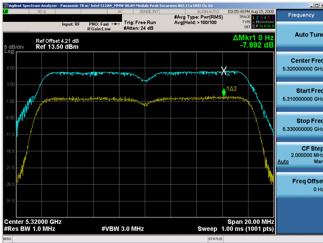
Plot 6-38. Peak Excursion Ratio Plot (802.11a (UNII) – Ch. 64)
