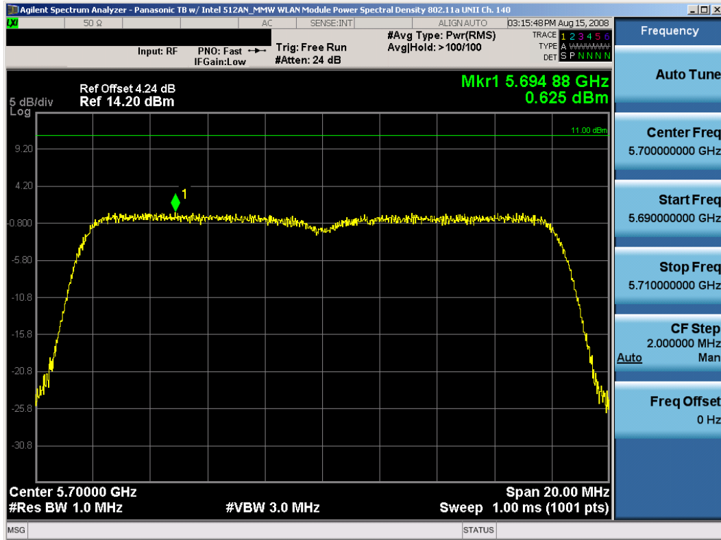
Plot 6-25. Peak Power Spectral Density Plot (802.11a (UNII) – Ch. 140)
