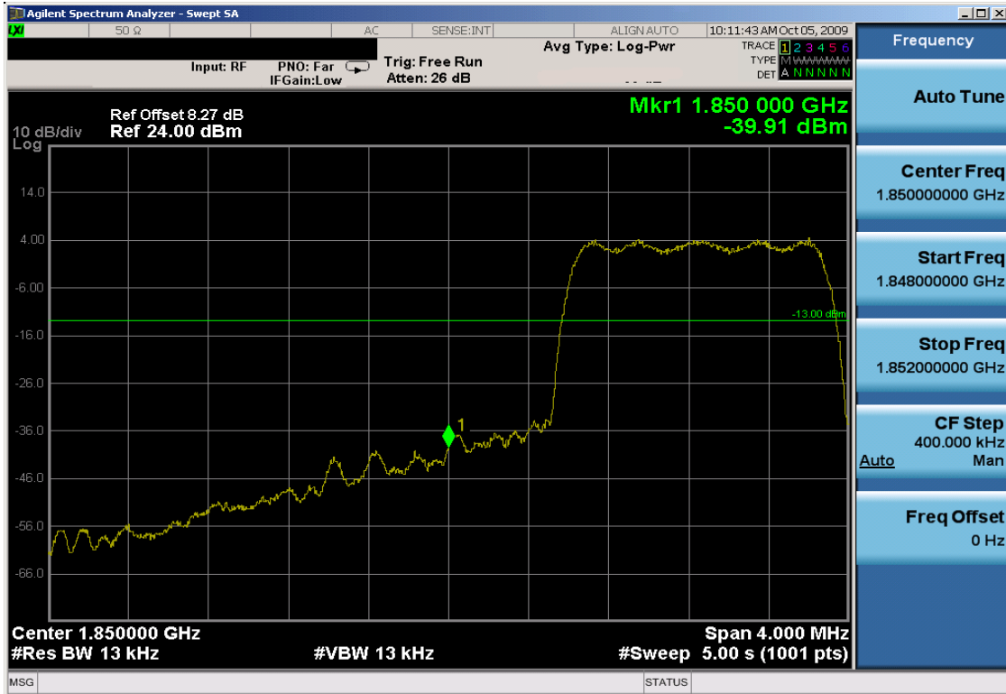
Plot 7-59. Band Edge Plot (PCS CDMA Mode – Ch. 25)
