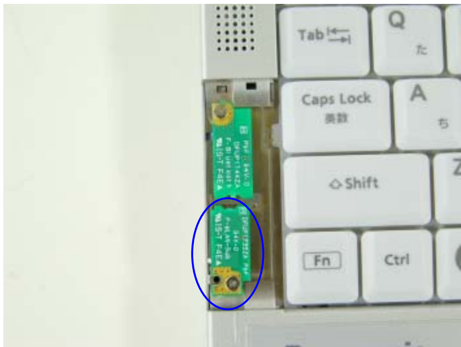
WLAN AUX TX/RX Antenna
