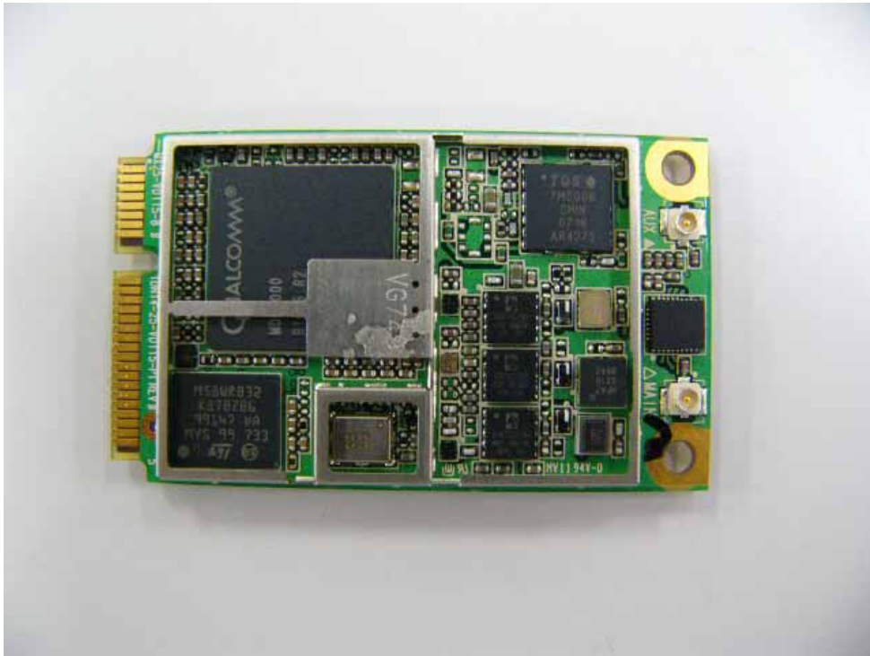
WWAN Module Interior Top View
