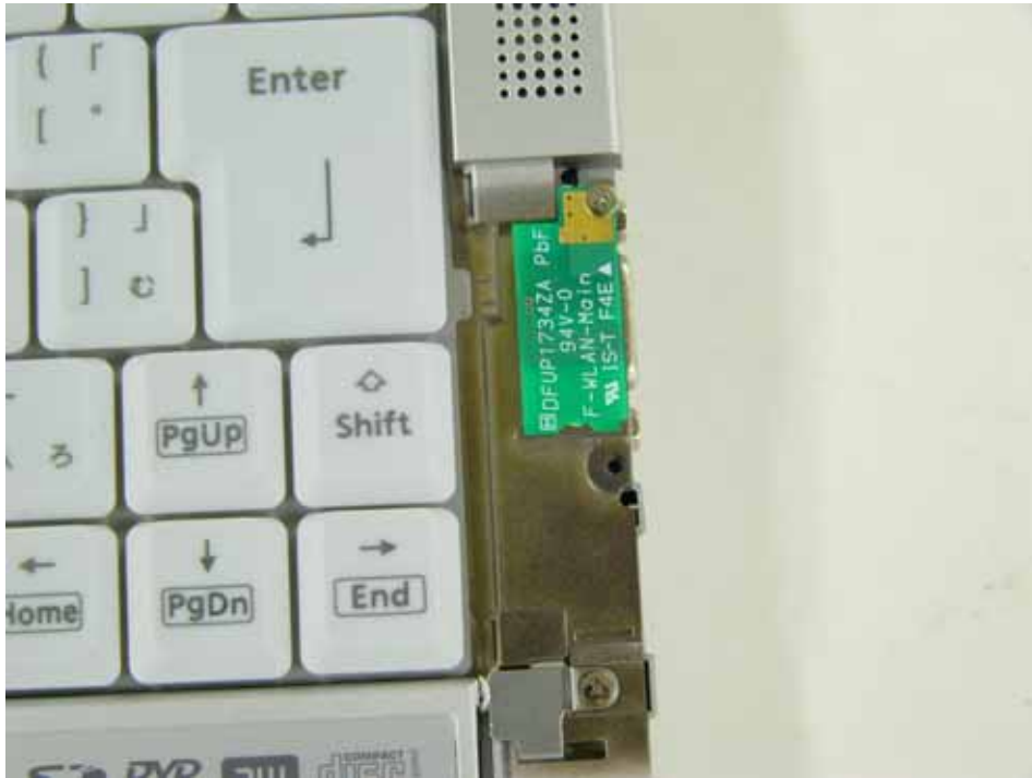
WLAN Main TX/RX Antenna
