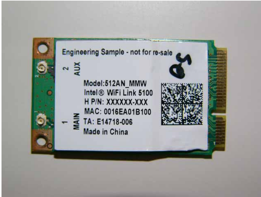
WLAN Exterior Top View
