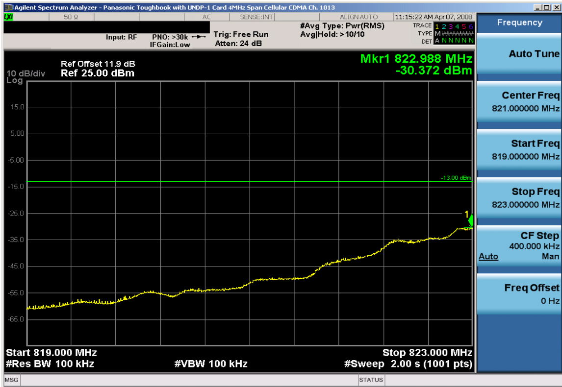
Plot 7-49. 4MHz Span Plot (Cellular CDMA Mode – Ch. 1013)
