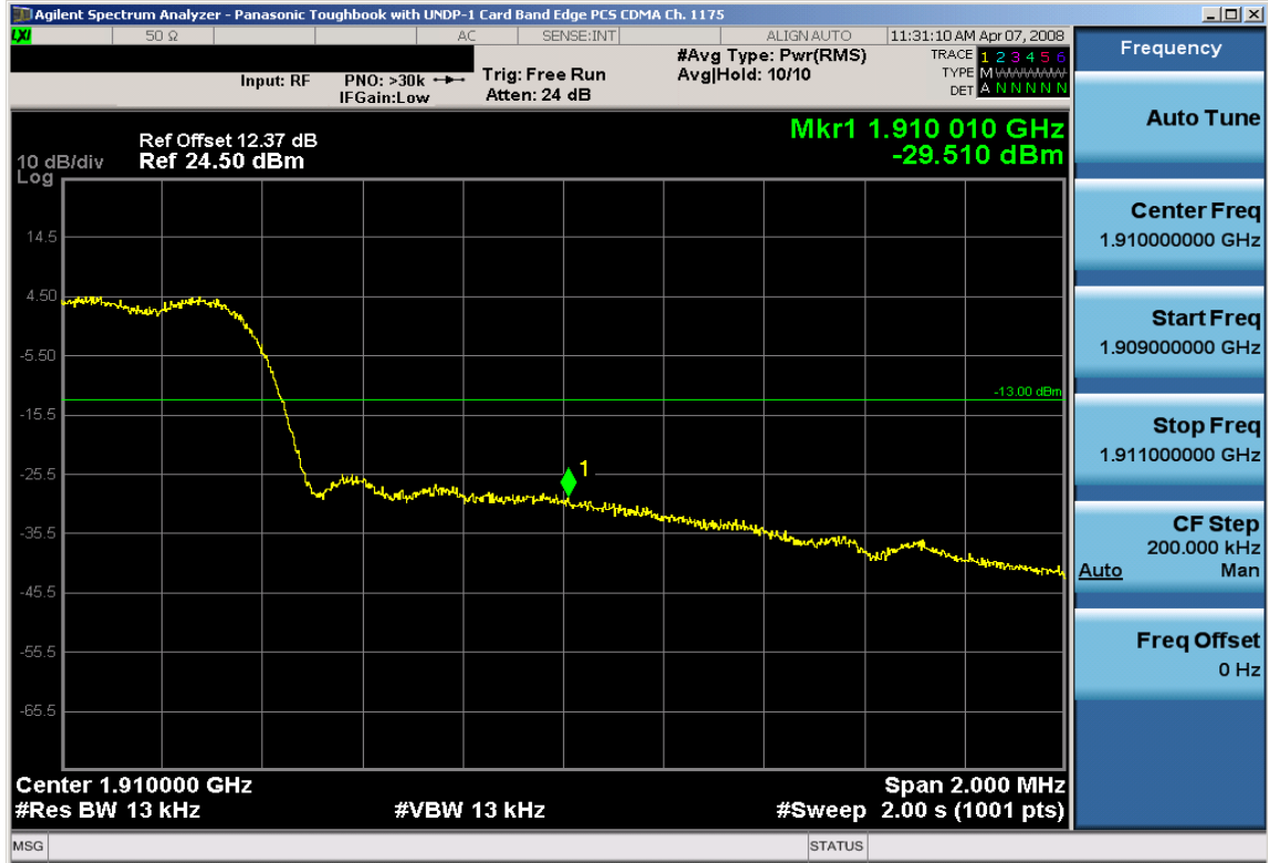
Plot 7-67. Band Edge Plot (PCS CDMA Mode – Ch. 1175)
