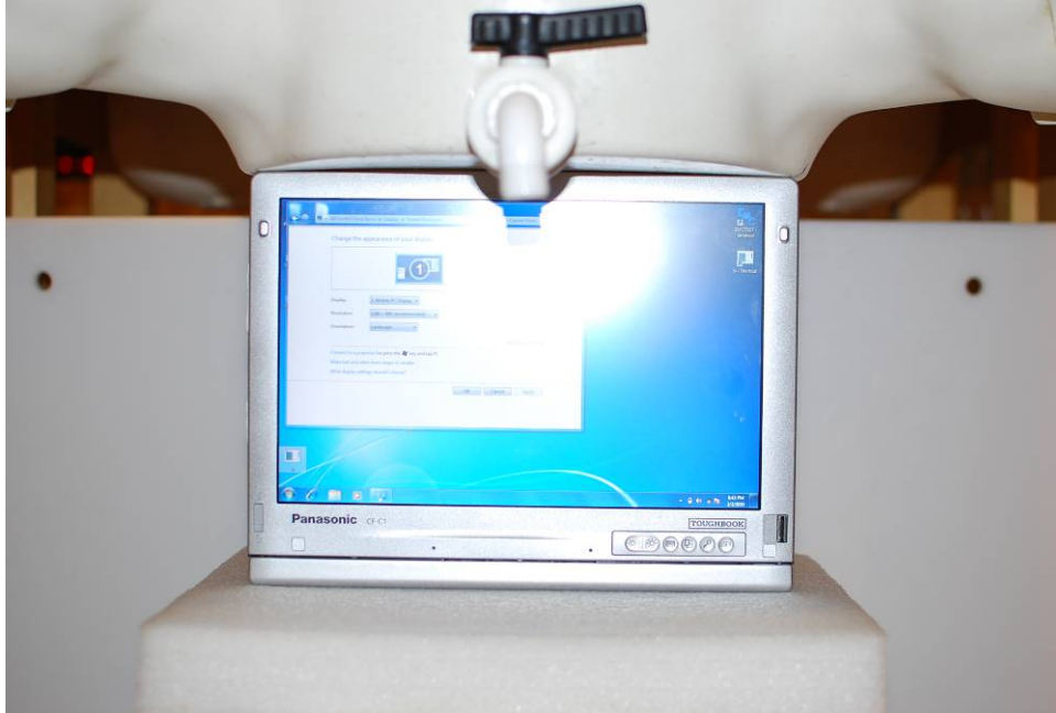
Figure 19-3 SAR Test Setup Photo 3: Edge Top
