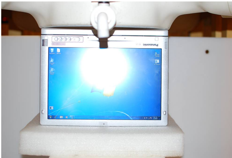
Figure 19-4 SAR Test Setup Photo 4: Edge Bottom
