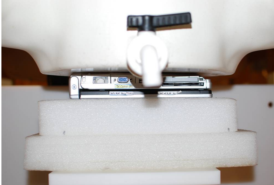
Figure 19-1 SAR Test Setup Photo 1: Laptop WLAN Antenna B (Left)
