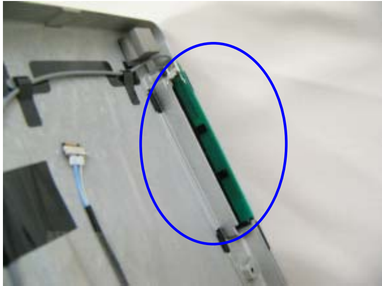
WWAN Main TX/RX Antenna
