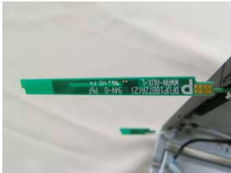
WWAN Aux RX Antenna Magnified view (Top)
