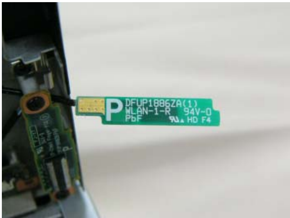
WLAN Main TX/RX antenna magnified view (Top)
