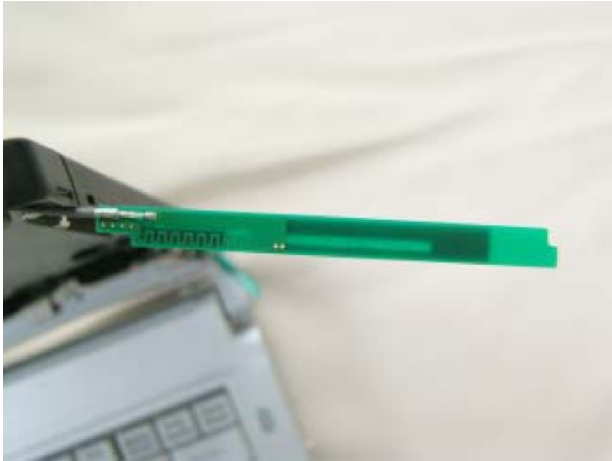
WWAN Main TX/RX Antenna magnified view (Bottom)
