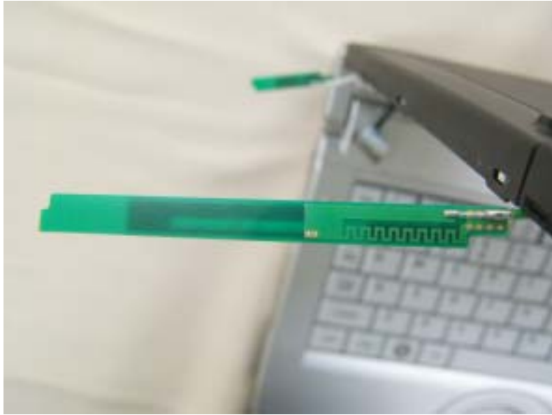
WWAN Aux RX Antenna Magnified view (Bottom)
