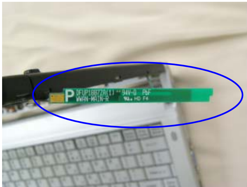
WWAN Main TX/RX Antenna magnified view (Top)
