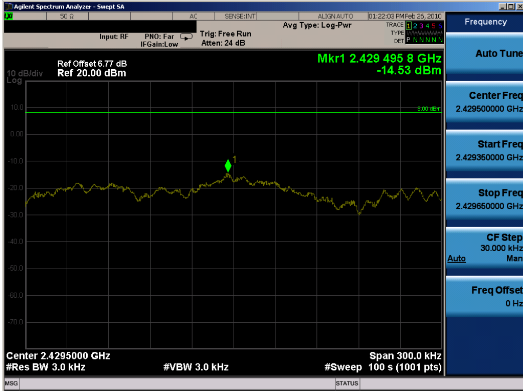
Plot 6-25. Power Spectral Density (802.11n (2.4GHz) Dual Transmit Mode – Ch. 6) – Chain A
