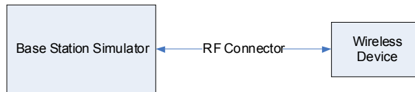
Figure 13-1 Power Measurement Setup
