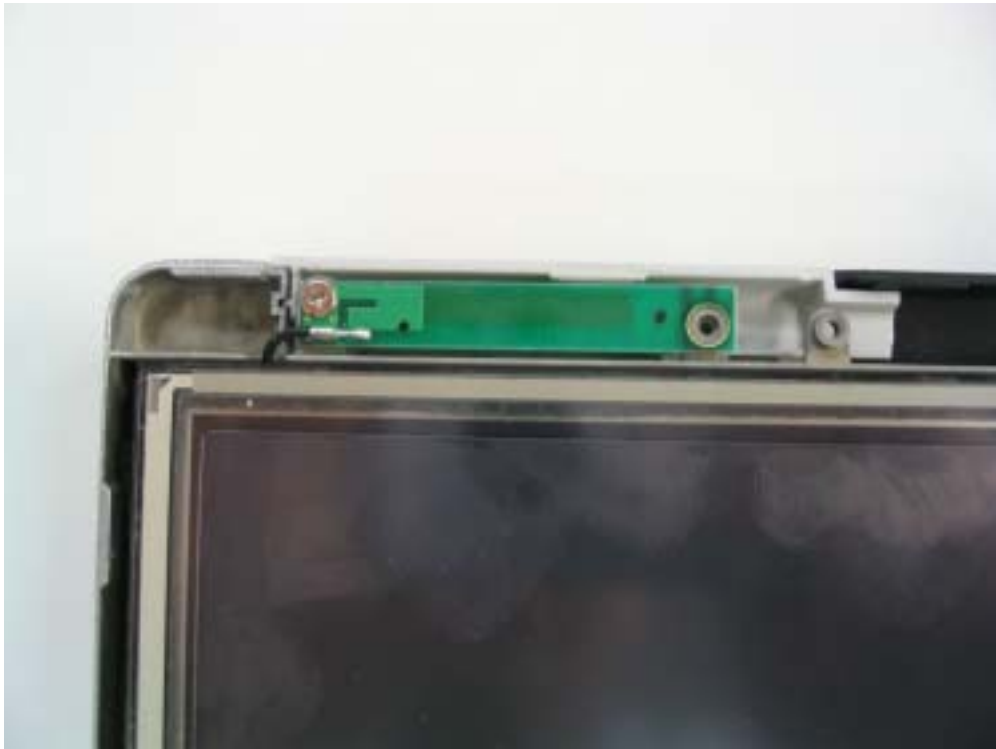
WLAN Main antenna magnified view
